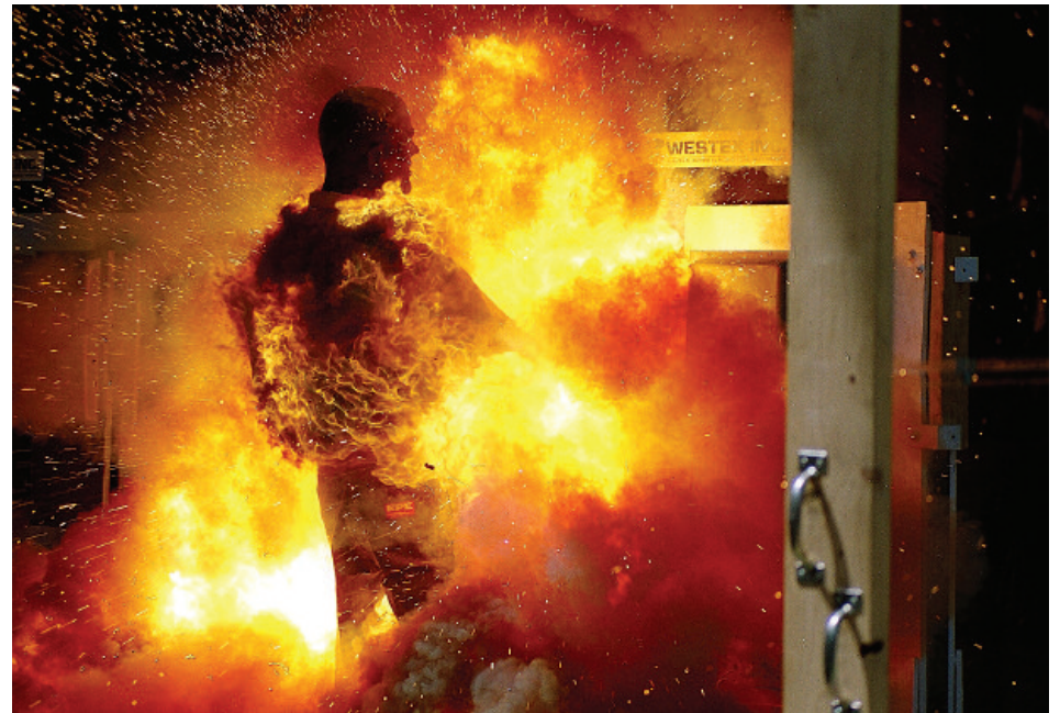
A still from a safety training video shows what can happen during an arc flash explosion.
