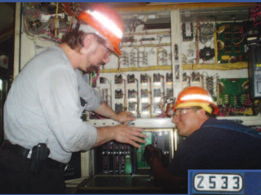
Local 912 member Fred Chesnes, left, trains member John Coleman on troubleshooting feedback circuits on a locomotive.
